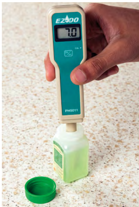
FIGURE 5.1.1 A pH meter is calibrated by measuring a series of reference standards, known as pH buffers, that have known and accurate pH values.
